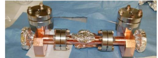
Example of 26 GHz dielectric loaded structures for two-beam-acceleration experiment:
