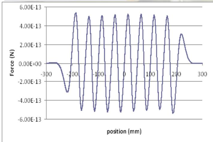
Making the end cell roughly half the length causes the field to cancel removing the offset. Similar work on 2 cell cavities was performed at ANL.
