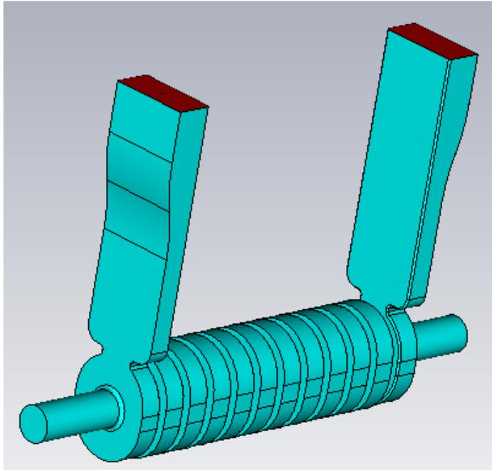
The structure being built for high gradient test at CERN has only a single feed as it will not see beam.
