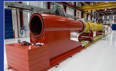
final cryomodule assembly
