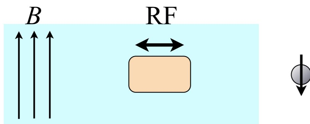
RF magnetic field in gradient field gives/removes the energy with spin flip.
