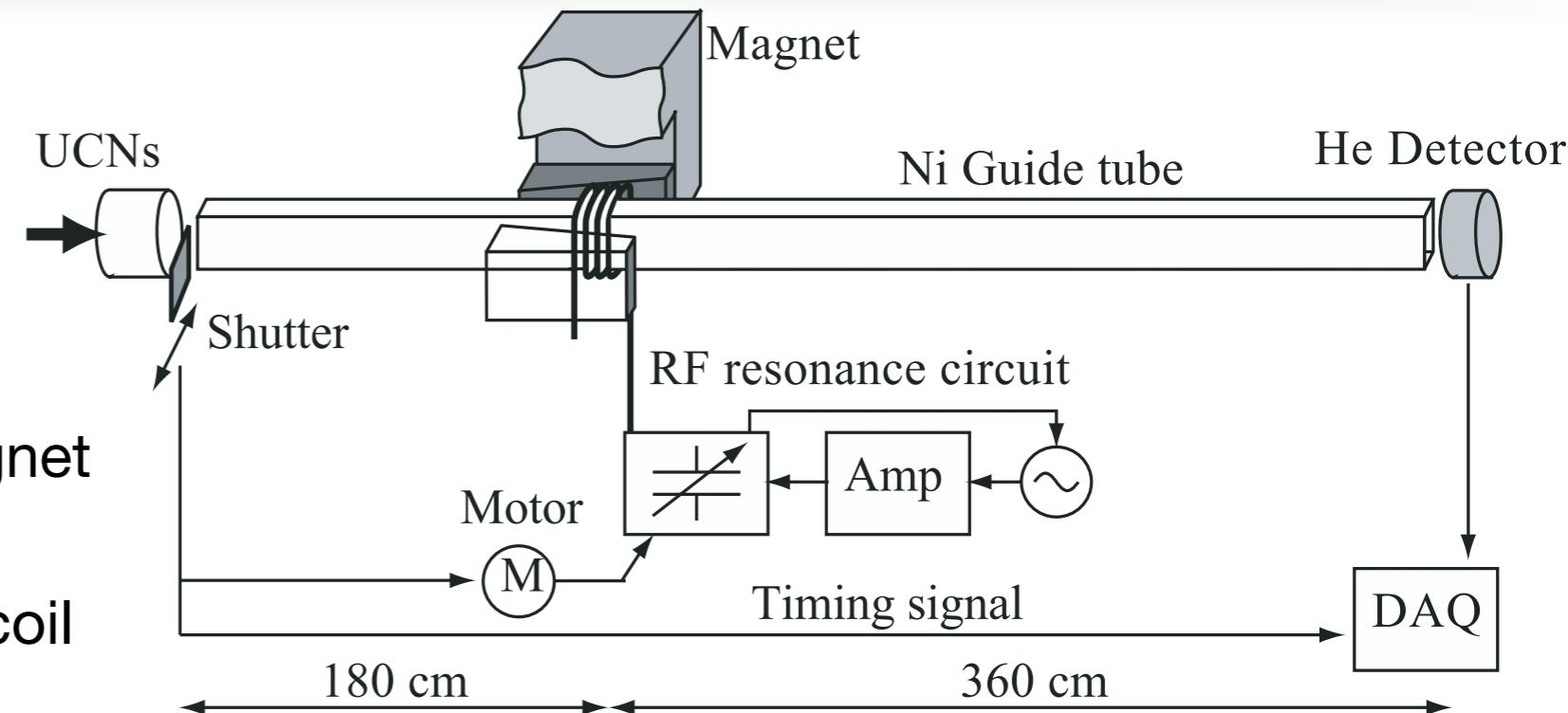
Continuous UCN beam was chopped by shutter to simulate **pulsed source**.
