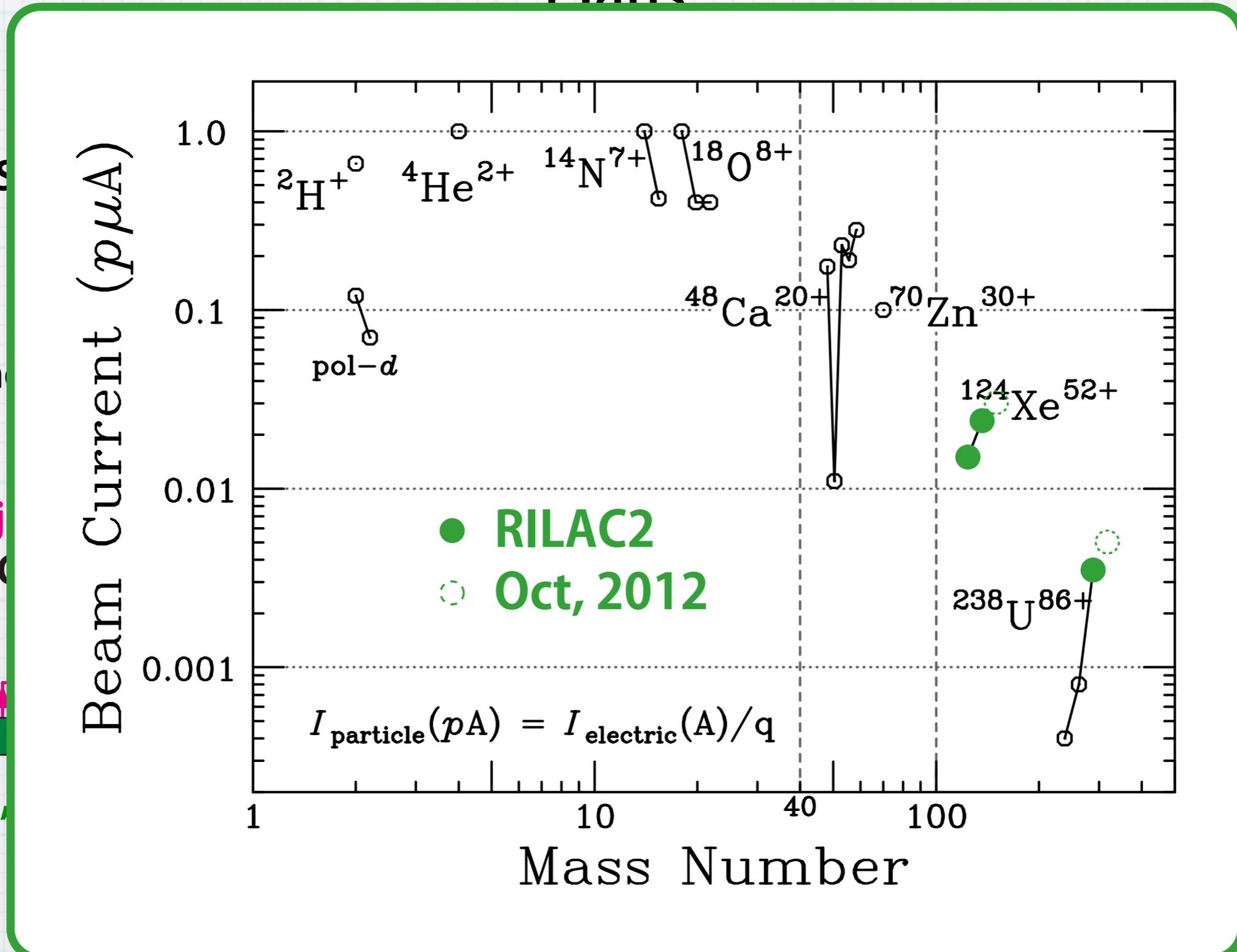
Beam current(Oct- , 2012):  $^{238}\text{U} > 5 \text{ pA}$ ,  $^{124}\text{Xe} > 30 \text{ pA}$
