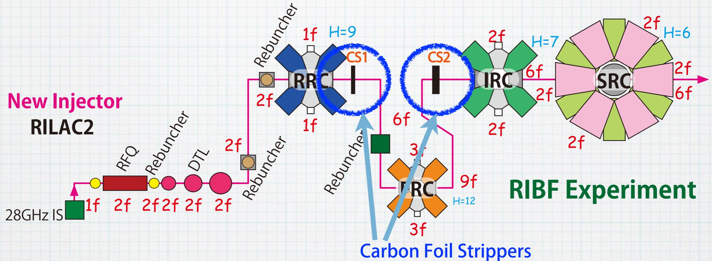
1. Cyclotron Cascades consist of RRC, and new booster cyclotrons with an injector linac.
