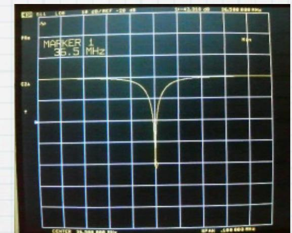
Resonant frequency  $f_0$  : 33.8 MHz  $\rightarrow$  36.5 MHz
