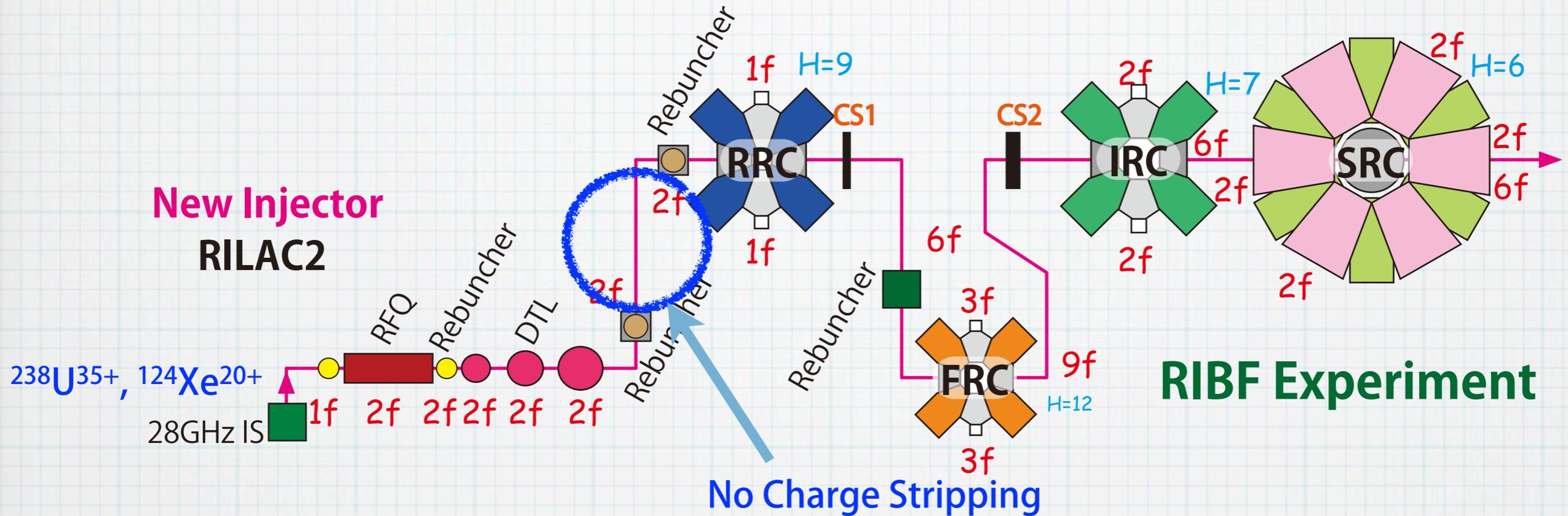
1. Cyclotron cascades consist of RRC, and new booster cyclotrons with an injector linac.
