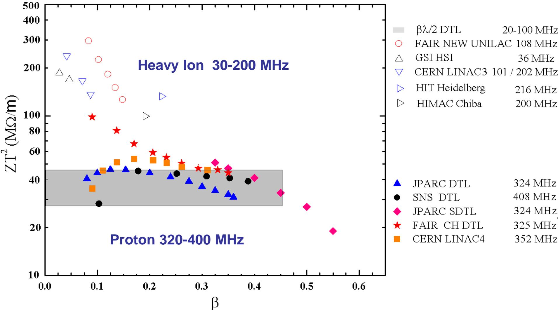
**IH-DTL Established as standard solution for Heavy Ion**
