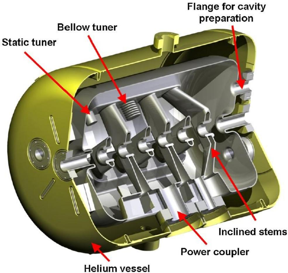
325 MHz, s.c. CH-DTL 5MV/m
