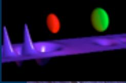
The first laser beam creates the accelerating structure, the second one is used to heat electrons
