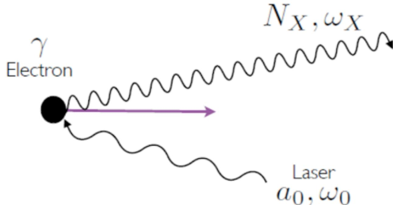
Doppler upshift : high energy photons with modest electrons energy :  $\omega_x = 4\gamma^2\omega_0$
