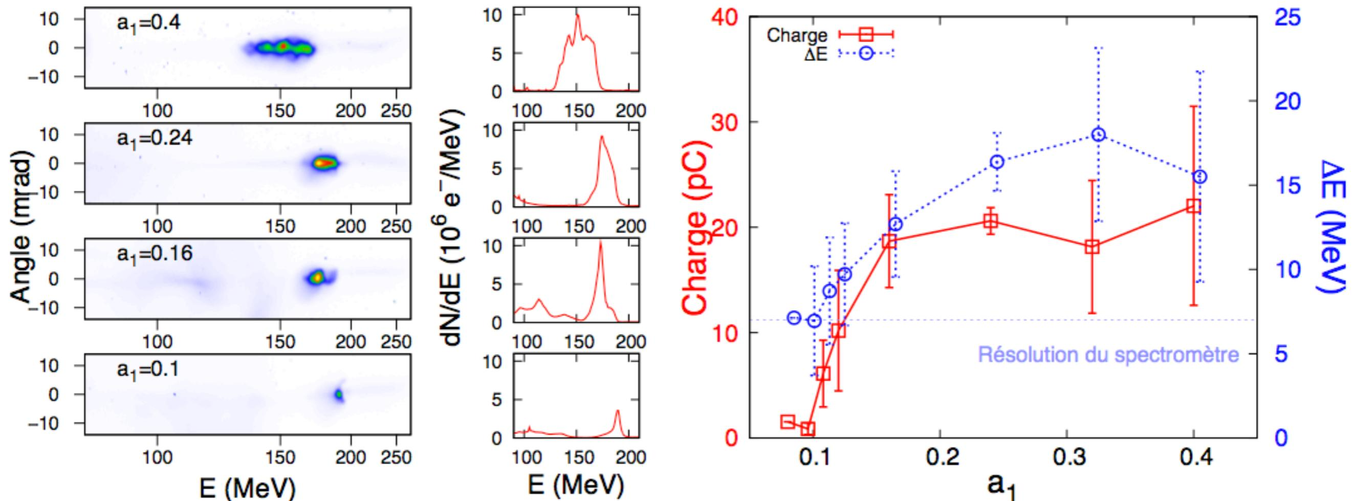
Charge from 60 pC to 5 pC,  $\Delta E$  from 20 to 5 MeV
