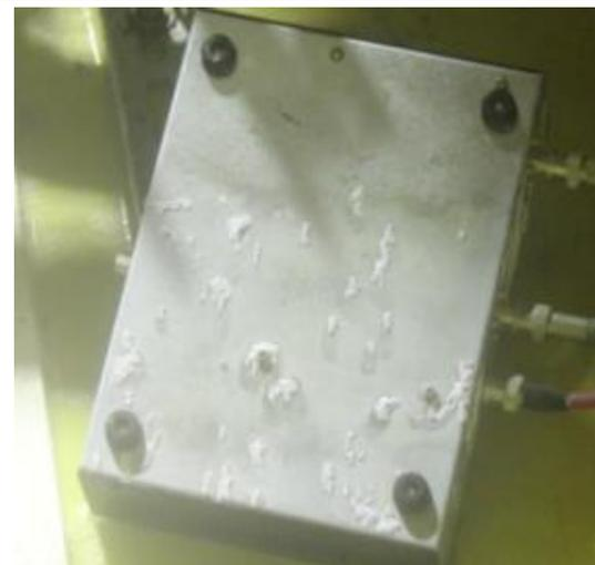
Corroded pre-amplifier boxes on the floor by strong alkaline.
