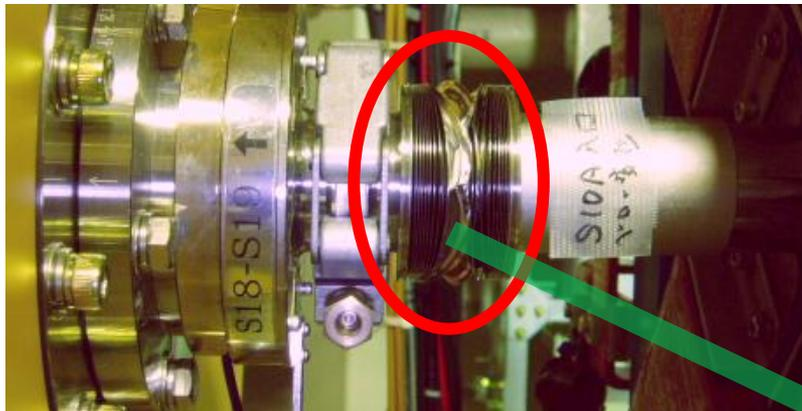
Distorted bellows between SDTL tanks
