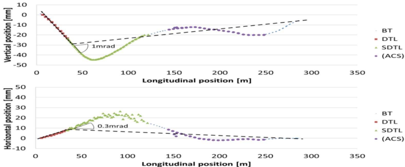
Displacement of components and target realignment line (dotted line)<sup>28</sup>
