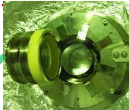
Broken current transformer: separated brazed ceramic parts and stainless parts
