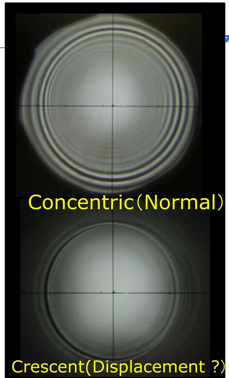
Inner view of the bore of the DTL by an alignment telescope.
