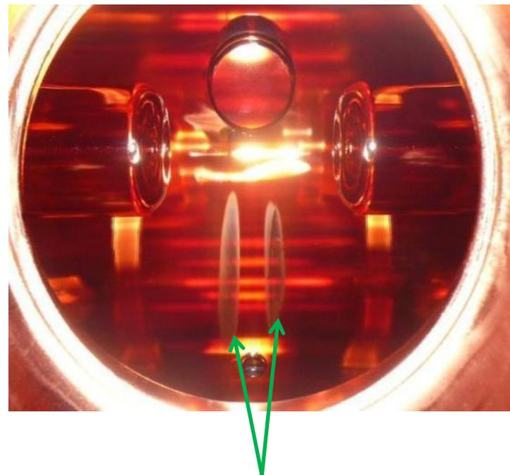
Inside view of the SDTL#5B cavity. Color change bands can be seen.
