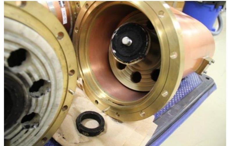
Loose connection of the coaxial line at the SDTL.
