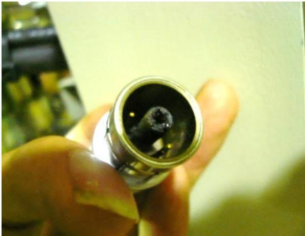
Discharge at the Ion Pump connector at the SDTL9B
