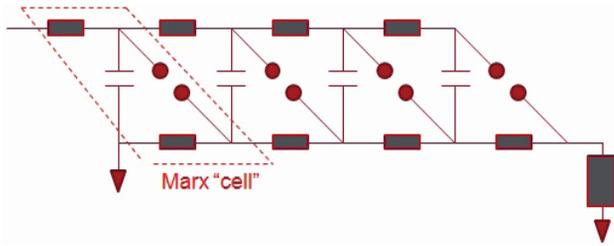
Fig. 1. Simple schematic of a capacitor-based Marx generator.
