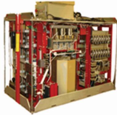
Figure 2. Photograph of the DTI ILC Marx Modulator.
