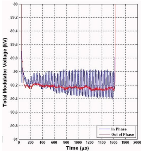
Figure 5. Measured output voltage for the SLAC P2 Marx. Shown is the output with the cells in phase and out of phase.
