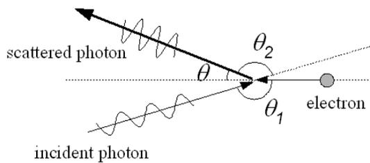
Figure 1: Laser Compton scattering.
