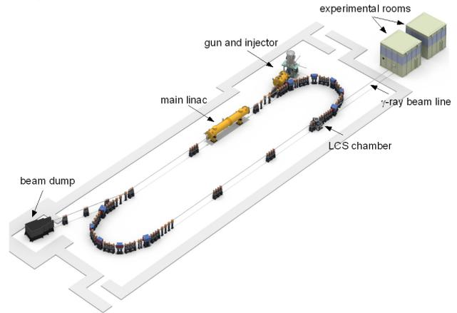
Figure 2: A schematic view of the LCS  $\gamma$ -ray experiment at the Compact ERL
