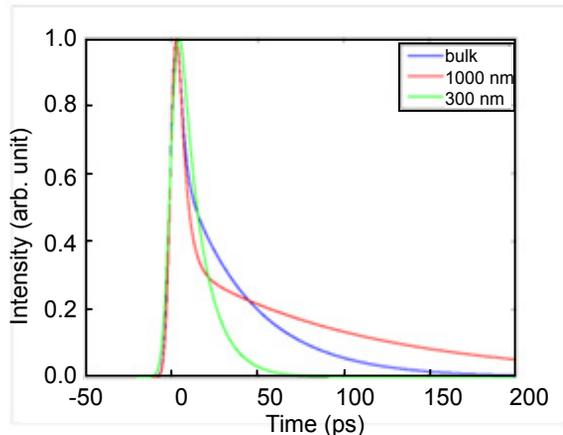
Figure 3: Temporal response of NEA GaAs photocathode by irradiation of short laser pulses ( $\sim$  ps,  $\lambda = 785$  nm) to a thickness of 300 nm, 1000 nm and bulk sample.
