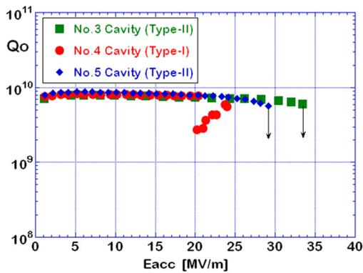
Figure 6: Final vertical test results of three 2-cell cavities with five RF feedthroughs (Type-I or Type-II) for five HOM couplers.
