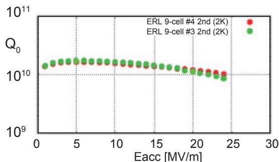
Figure 7: Q-E plot of the 9-cell cavities for the cERL main linac module.
