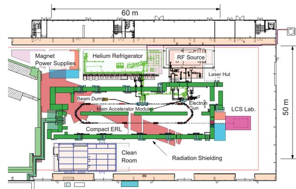
Figure 9: Current plan of the Compact ERL for commissioning.
