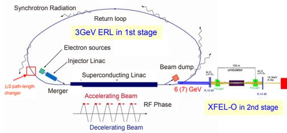
Figure 1: Conceptual layout of 3-GeV ERL plan integrated with an X-ray free electron-laser oscillator (XFEL-O).
