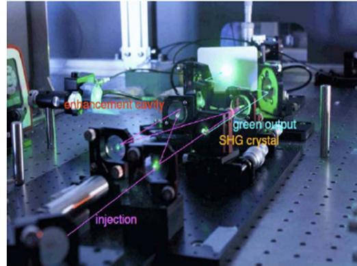
Figure 4: Laser system with cavity wavelength conversion.
