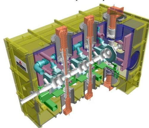
Figure 5: Schematic drawing of the injector cryomodule containing three 2-cell cavities and six input couplers.
