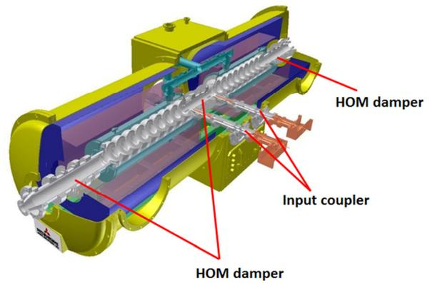
Figure 8: Schematic drawing of the prototype module of the cERL main linac. A pair of 9-cell cavities is connected with LN<sub>2</sub>-cooled HOM dampers.
