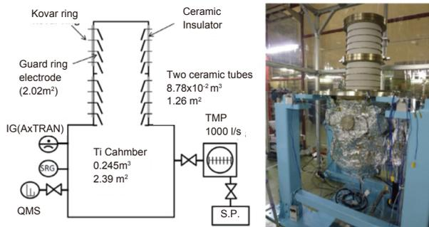
Figure 2: Layout of the vacuum system for the 2<sup>nd</sup> gun at KEK (left), and a photograph of the system (right).
