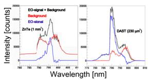
Figure 3: First BCD measurements with 230-µm thick organic DAST crystal compared with EO signals with a 1-mm inorganic ZnTe crystal. The both of the crystals were set 2.0 mm from the electron beam axis.
