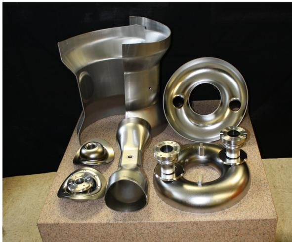
Figure 3: The niobium subassemblies which will be welded together to make the HWR. The parts clockwise from top left are outer-conductor halves, toroids, inner-conductor, and re-entrant noses.
