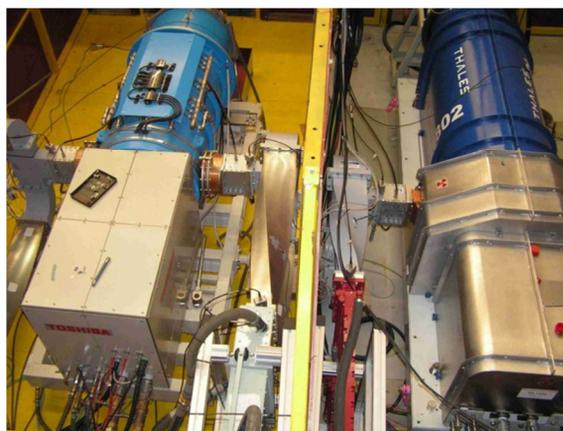
Figure 1: MBK test stands in DESY Hamburg
