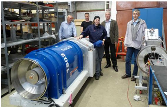
Figure 7: The first serial MBK for XFEL on DESY site.
