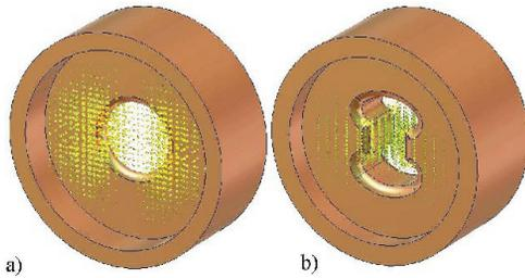
Figure 1: DLW (a) and TE - type (b) deflectors.
