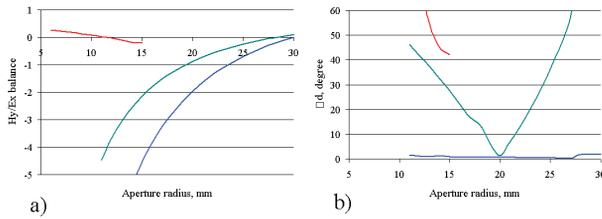
Figure 3: The field balance  $\frac{Z_0 H_y^0}{E_x^0}$  (a) and  $\Psi_d(a)$  plots (b) for DLW deflector  $\Theta_0 = 60^\circ$  (blue),  $\Theta_0 = 180^\circ$  (green) and TE - type deflector,  $\Theta_0 = 180^\circ$  (red).
