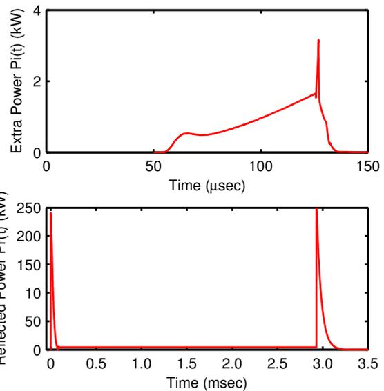
Figure 6: The extra incident power  $P_i(t)$  required to compensate the beam loading and the reflected power  $P_r(t)$  vs. time. Note that the time scales are different.
