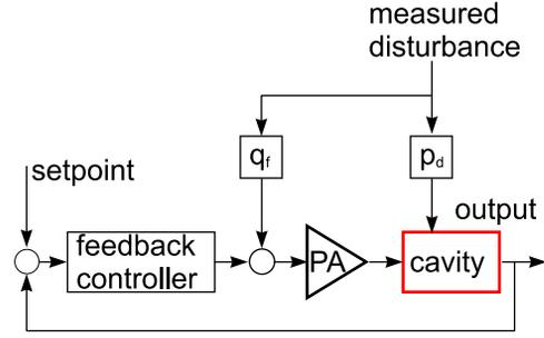
Figure 2: Feedback and feed-forward control of the accelerating voltage of a cavity fed by a power amplifier (PA).
