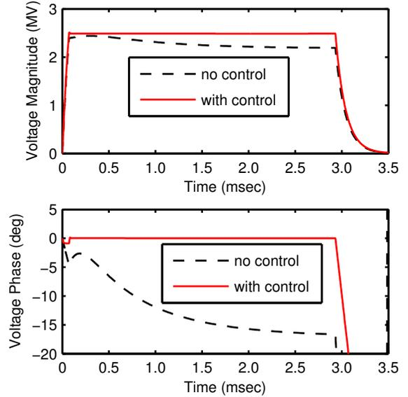
Figure 3: The cavity voltage magnitude and phase vs. time. The solid red curves stand for the spoke cavity with the implemented feedback and feed-forward control whereas the dashed black curves stand for the case with no control.
