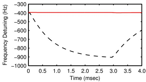
Figure 4: Dynamic detuning of the frequency caused by the electromagnetic pressure vs. time. The red solid curve and the black dashed curve stand for the cavity with and without control, respectively.
