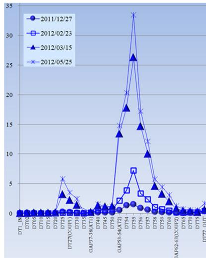
Figure 4: Residual Radiation at DTL1. Radiation depends on the operation history and beam outputs. Unit of longitudinal axis is in μSv/h and horizontal axis describes the position.
