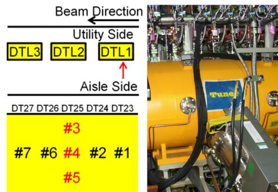
Figure 3. Measurement Points of 1st DTL1 Cavity. Axis is defined to the x-y-z coordination, +y as a top of vertical, +z as a beam direction, +x as a inevitably defined for aisle direction.
