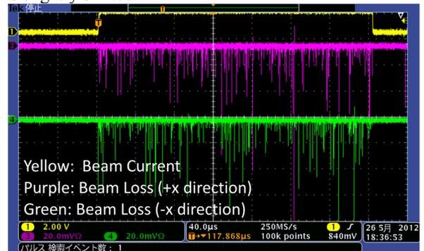
Figure 9: Beam Loss Events Occurred at DT55. Beam orbit is corrected with observing beam losses occurring from DTL to downstream section.
