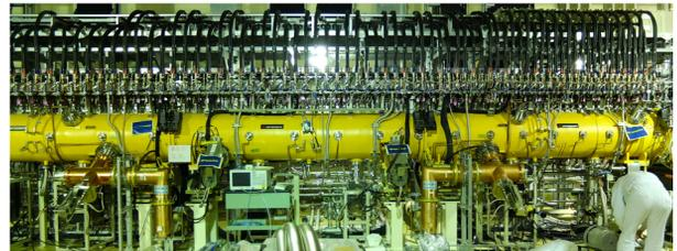
Figure 2: Overview of DTL Cavity. One DTL cavity consists of 3 unit tanks.
