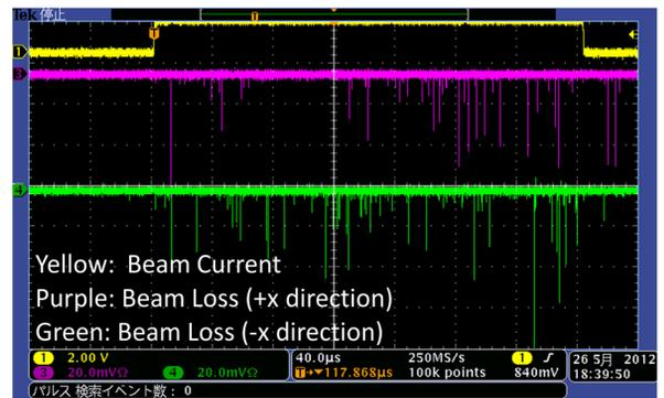
Figure 7: Beam Loss Events Occurred at DT25. Beam orbit is corrected with observing beam losses occurring from DTL to downstream section.
