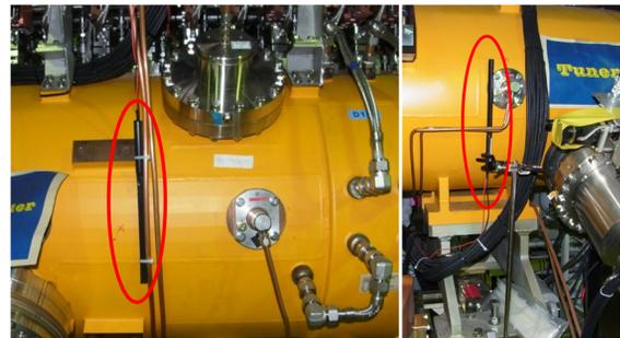
Figure 6: Scintillation BLMs Installed at the Surface of DTL Cavity. Installation situation of DT25 is on left side and it of DT55 is on right side.
