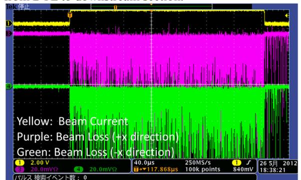
Figure 10: Beam Loss Events Occurred at DT25. Many beam loss events are observed, after the beam orbit is slightly shifted.
