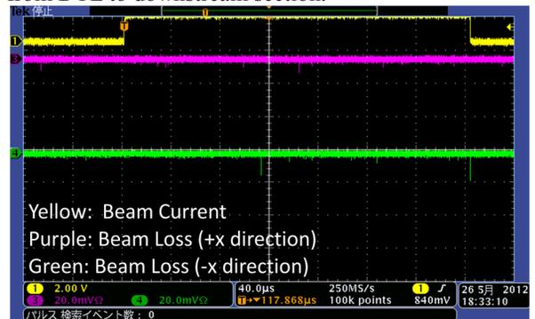
Figure 8: Beam Loss Events Occurred at DT25. Many beam loss events are disappeared, after the beam orbit is slightly shifted.
