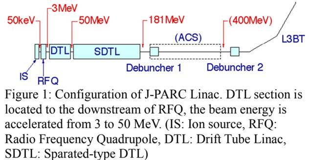
Figure 1: Configuration of J-PARC Linac. DTL section is located to the downstream of RFQ, the beam energy is accelerated from 3 to 50 MeV. (IS: Ion source, RFQ: Radio Frequency Quadrupole, DTL: Drift Tube Linac, SDTL: Separated-type DTL)
