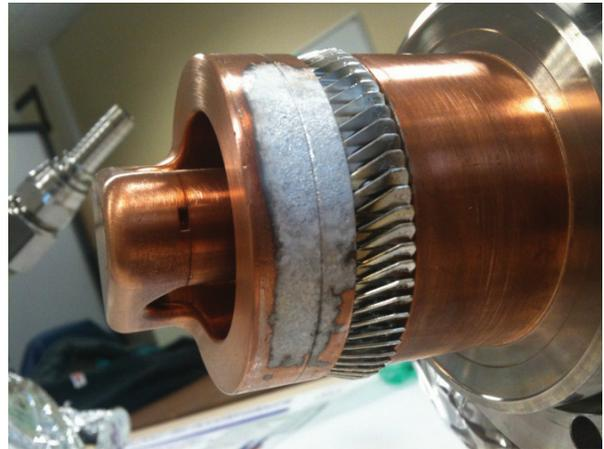
Figure 5: Particular of the coupler after the tests: the aluminum sputtering on the copper surface and the damaged spring contact are visible.
