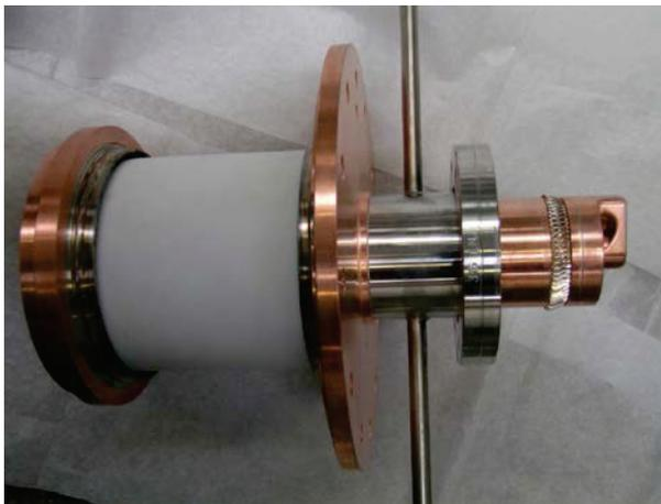
Figure 1: RF coupler system with loop, coaxial transmission line and coaxial alumina window.
