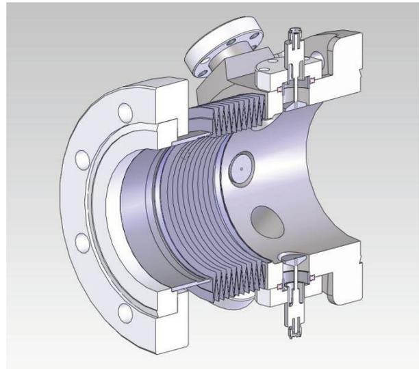
Figure 1: A cross-section view of the button BPM.
