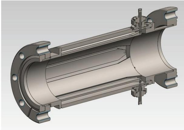
Figure 2: A cross-section view of the stripline BPM.
