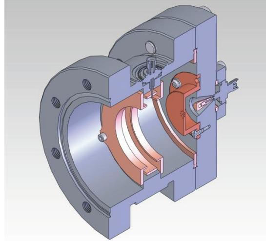
Figure 5: A cross-section of the capacitive and coaxial pickups assembly.
