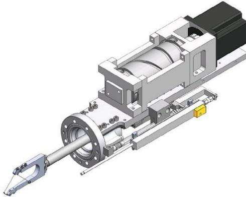
Figure 4: The preliminary design of the fast wire scanner.
