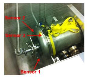
Figure 4: Setup for the preliminary cold test. Thermal sensors on top, alongside and bottom of the end cap.
