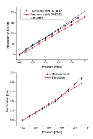
Figure 7: Top: Frequency shift due to evacuation. Bottom: Deformation of the cavity quarter shell versus residual pressure.
