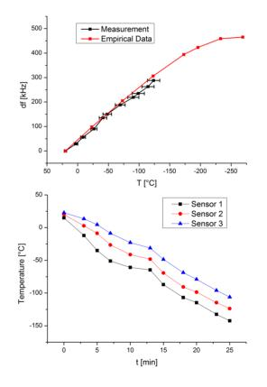
Figure 5: Top: Measured and expected frequency shift due to thermal shrinkage (Empirical data taken from: A.F. Clark, Materials at Low Temperatures). Bottom: Temperature behaviour for all three sensors.
