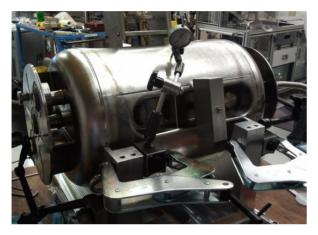
Figure 6: Setup for pressure sensitivity measurement.
