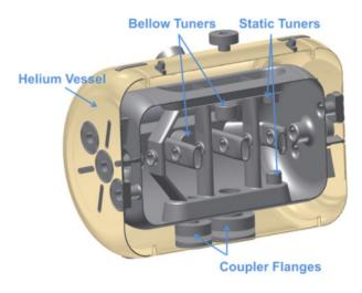
Figure 1: Layout of the superconducting 7-cell CH-Cavity (325.224 MHz,  $\beta = 0.16)[4]$ .
