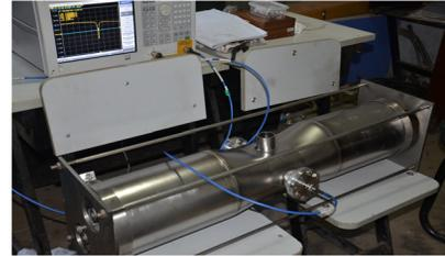
Figure 6: Frequency measurement before final welding.
