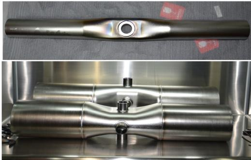
Figure 5: The main parts of IMP HWR.
