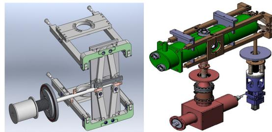
Figure 3: Tuner and HWR assembled with coupler and tuner.
