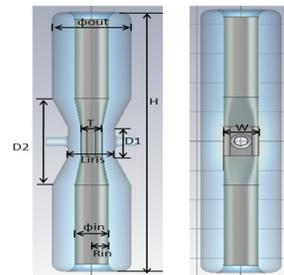
Figure 1: Parameters of the cavity geometry used in the RF optimization.
