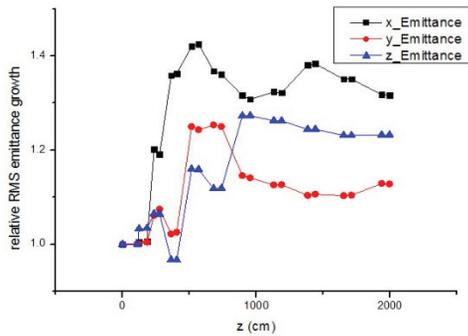
Figure 6: The relative emittance growth along the linac.
