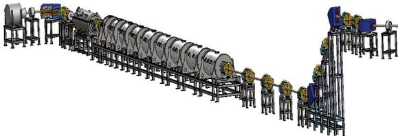
Figure 2: The 3-Dimensional Map of the heavy ion linac for CSRm.
