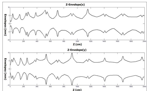
Figure 3: The x and y transverse envelope along the linac.
