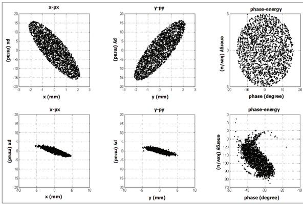
Figure 5: The phase space distribution at the entrance and exit of the DTL section.
