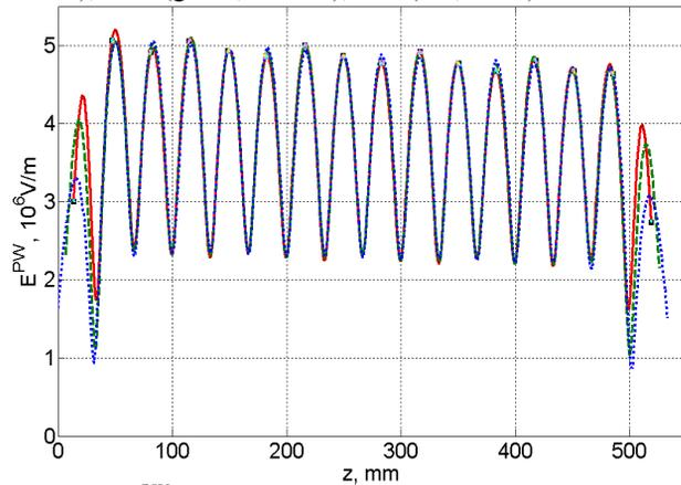
Figure 6:  $E^{PW}(z, x=a=4\text{mm})$  for different coupler lengths:  $D$  (blue, dotted),  $3D/4$  (green, dashed),  $D/2$  (red, solid).
