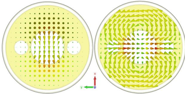
Figure 1: Electric (left) and magnetic (right) fields of TE<sub>11</sub> mode.
