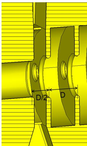
Figure 3: Coupler with length of  $D/2$ .
