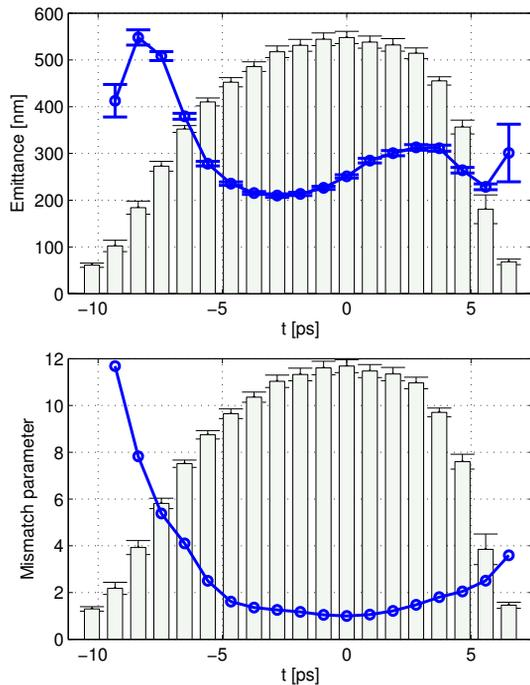
Figure 4: Slice emittance measurement at 200 pC: charge profile (bars) in comparison to slice emittance (top) and relative mismatch parameter (bottom) as a function of position along the bunch.
