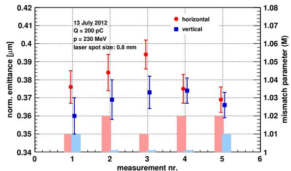
Figure 3: Stability of emittance measurement: the same single-quadrupole scan was repeated five times with 2 minutes between measurements. The measured emittance is shown in  $\mu\text{m}$  (left-hand scale), error bars are determined from the evaluation of 10 images per set point. Also shown (bars, right-hand scale) is the mismatch parameter determined by the fit to the optics as a measure for the matching quality (optimum value is 1).
