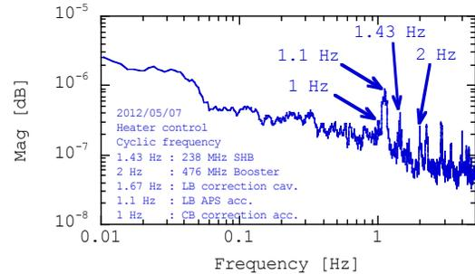
Figure 8: Spectrum of the beam position jitters after BC1 under different conditions of the operating cycle of the cooling water temperature controller in the RF cavity.
