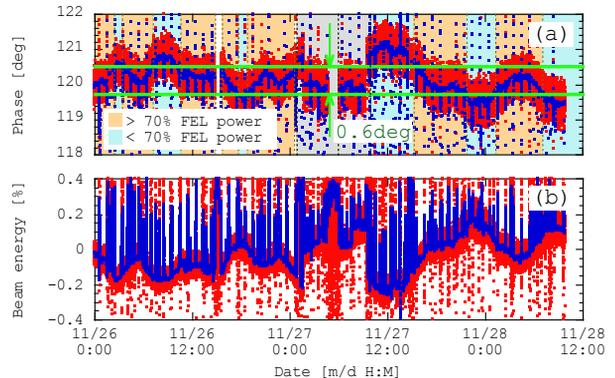
Figure 4: (a) Beam arrival time after BC1. The beam phase is equivalent to 0.58 ps/1 degree. (b) Beam energy in BC2, where the energy dispersion is  $\eta = -345\text{mm}$ .
