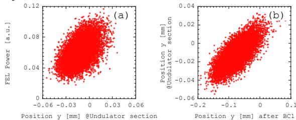
Figure 6: (a) Correlations between the beam position at the entrance of the undulator section and the laser power. (b) Correlations between the beam position after BC1 and at the entrance of the undulator section.
