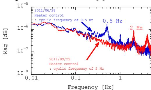
Figure 7: Results of a period analysis using the beam position jitters data after BC1. Blue and red lines are the spectra when the temperature controller of RF cavities was operated at a cycle of 0.5Hz and 2Hz for the heating regulation, respectively.
