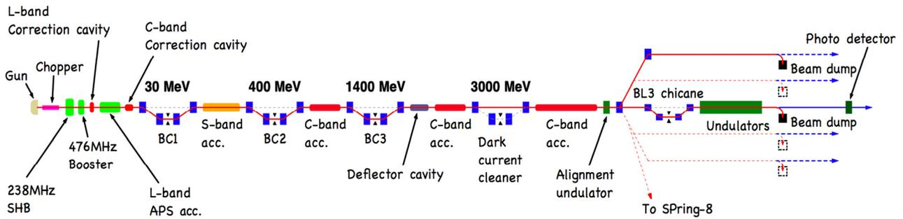
Figure 2: Schematic view of the linear accelerator and undulator section in SACLA.
