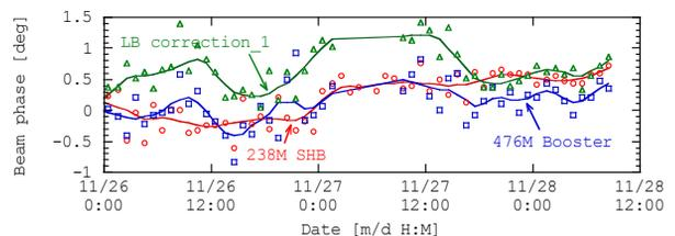
Figure 5: Beam arrival time obtained by an induced voltage from the beam in each RF cavity of the injector.
