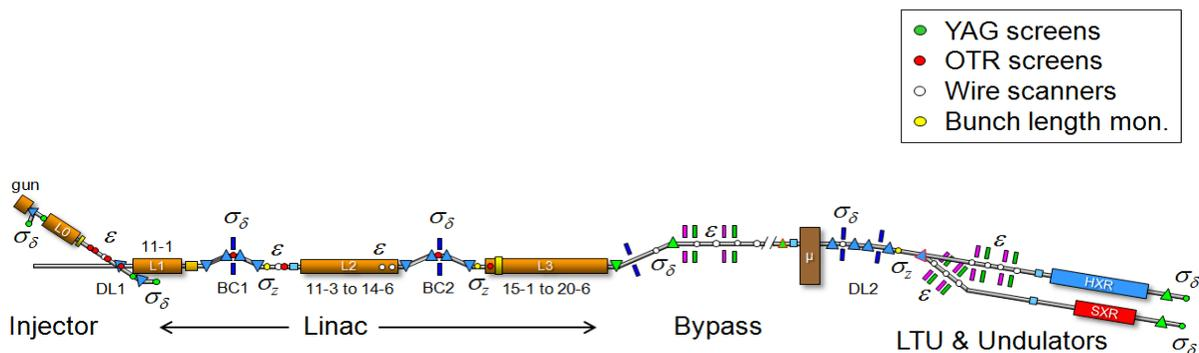
Figure 3: Schematic of the LCLS-II design illustrating the Injector, Linac and bunch compressors, the 1.2 km long bypass around LCLS-I and the Linac-to-Undulator (LTU) and undulators. The primary beam diagnostics are shown for each section.
