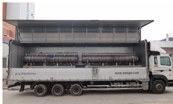
Figure 5: 20-MeV DTL tanks on the vibration free truck for the movement to Gyeongju site
