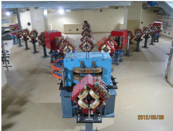
Figure 7: The installed 20-MeV beam line magnets in the 20-MeV beam line hall
