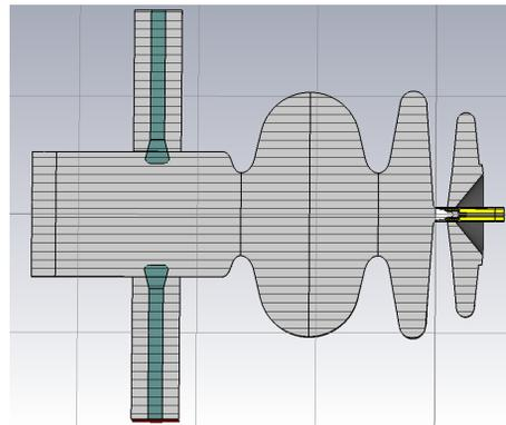
Figure 5: Possible design of the next 1.4 cell gun cavity featuring the HZDR-style choke cell, a modified cathode, two TTF-III type FPC having a 35 mm exit iris.
