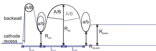
Figure 1: Geometry design parameters used for the cavity optimization scheme.
