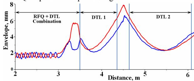
Figure 3: Calculated envelopes of  $^{12}\text{C}^{4+}$  – ions at 10 mA for x (blue curve) and y (red curve) planes.
