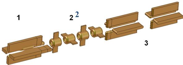
Figure 2: 3D model of the RFQ output part: 1 – the end of regular RFQ vanes, 2 - drift tubes, 3 - rf quadrupoles.
