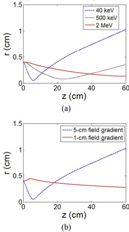
Figure 2: Beam envelope for (a) different injection energies, (b) two different lengths of field gradient at the DWA entrance for a 40-keV proton beam.
