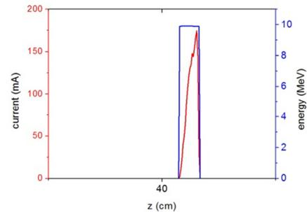
Figure 7: Proton energy and current profile at the exits of the DWA (with screen).
