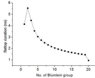
Figure 6: Electric pulse flattop duration as a function of the No. of HGI group.
