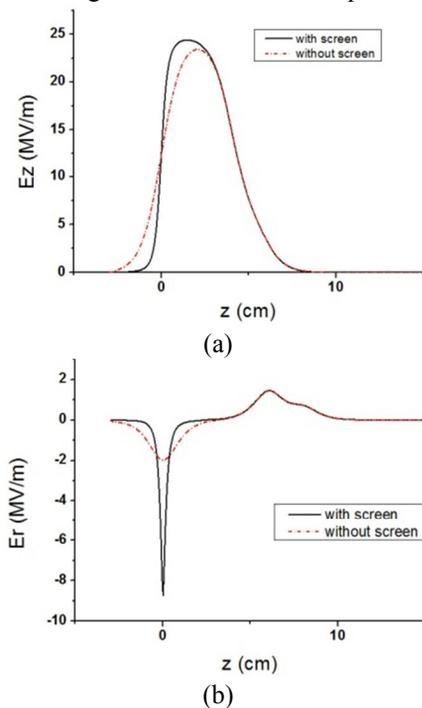
Figure 4: Longitudinal (a) and radial (b) electric field profiles at the DWA entrance with and without entrance screen.
