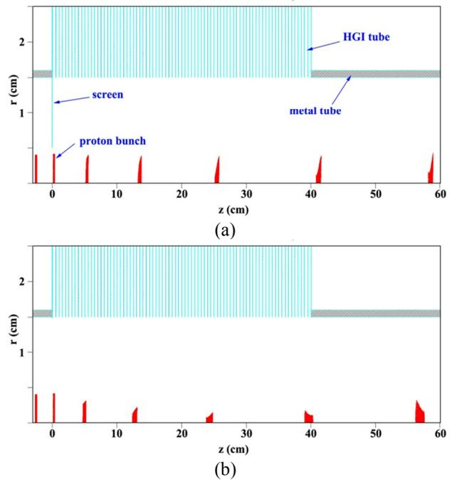
Figure 3: Beam transports in a 10-MeV DWA, (a) entrance screen can further reduce the focusing force at the entrance, (b) the proton bunch was over-focused when there was no entrance screen.
