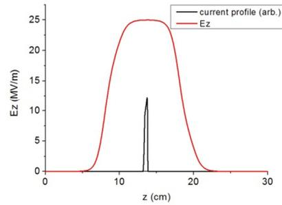
Figure 5: Longitudinal electric field and proton current profile in the middle of the DWA.
