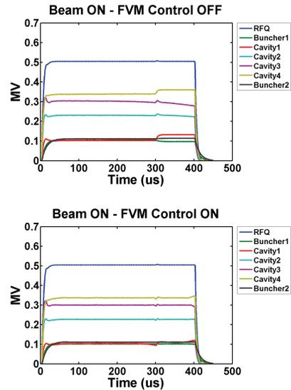
Figure 4: Cavity Magnitude with FVM LFF loops OFF/ON
