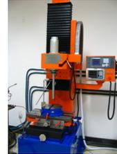
Figure 10: Rotating-coil magnetic measurement system.
