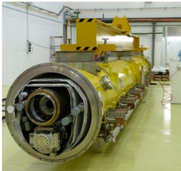
Figure 7 : CM after warm coupler assembly
