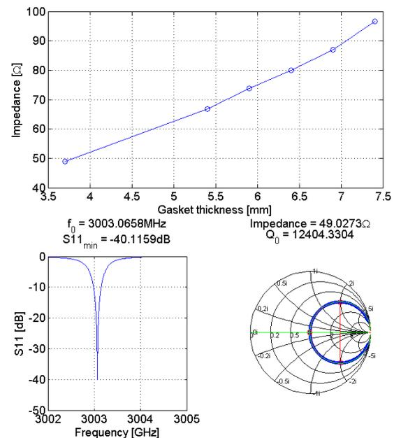
Figure 3: Tuning of gasket thickness for critical coupling (above) and cold test results at critical coupling (below).
