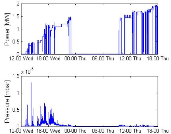
Figure 11: S-band gun conditioning
