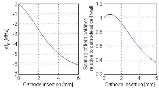
Figure 6: Prediction of cathode tuning
