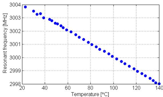
Figure 5: Scaling of resonant frequency with temperature before correction.
