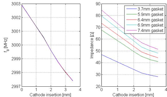
Figure 7: Change of resonant frequency (left) and impedance (right) with re-entrant cathode.
