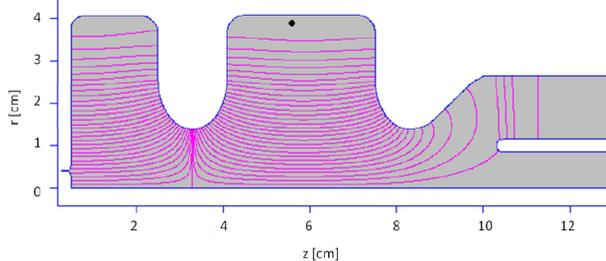
Figure 1: SUPERFISH calculation of  $\pi$  mode
