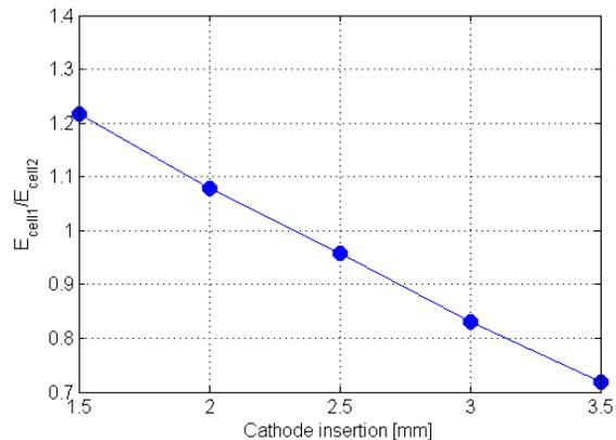
Figure 8: Field balance measurements with re-entrant cathodes.
