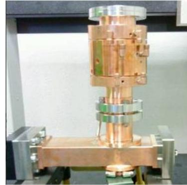
Figure 2: The assembled gun and coupler
