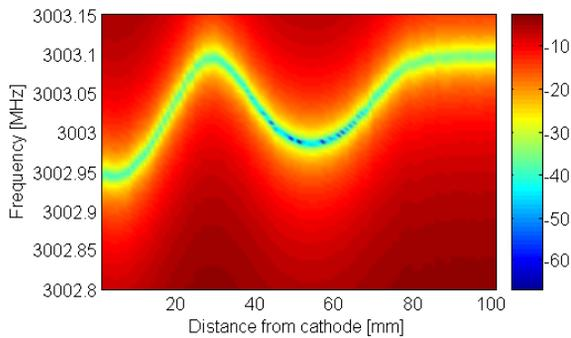
Figure 4: Bead pull results before correction
