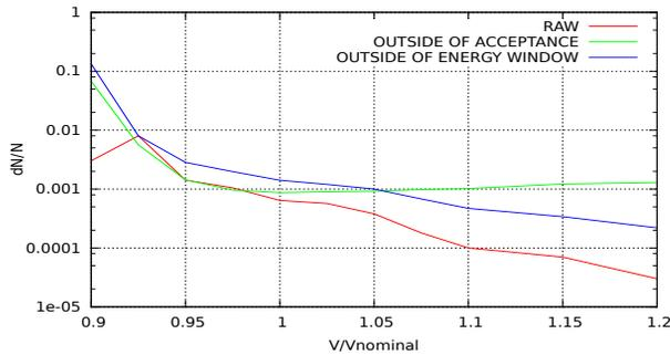
Figure 5: Estimated loss fractions vs relative voltage.
