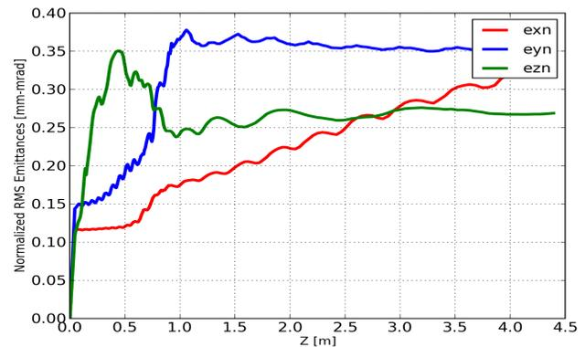
Figure 8: Emittances with 2 mm, 2 mrad vert. input error.
