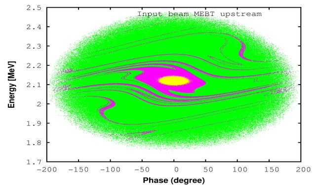
Figure 4: Longitudinal phase space acceptance for the combined MEBT and Linac. The acceptance is the cyan area. The yellow area is a  $3\sigma$  beam.
