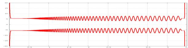
Figure 1: Vane profile in the horizontal plane.
