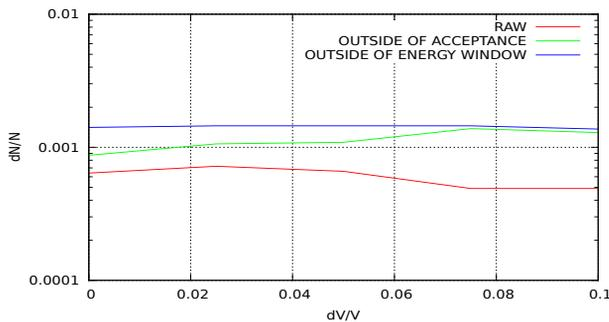
Figure 6: Estimated loss fractions vs linear voltage ramp.
