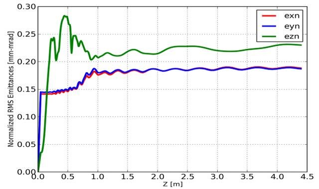
Figure 7: Emittances with a 50 % hor. input mismatch. Losses are not affected.
