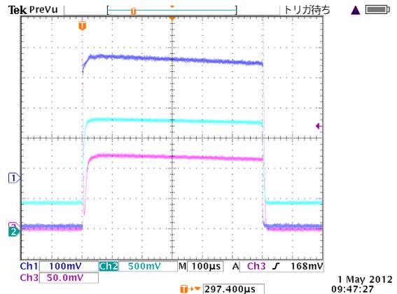
Figure 4: RF waveform of RFQ II. Blue: tank level, Cyan: inputted RF, Magenta: reflected RF.
