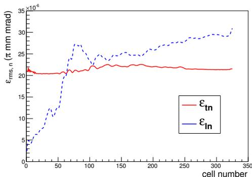
Figure 6: Emittance evolution as functions of cell number. The solid line represents the transverse normalized rms emittance, and the dashed line is the longitudinal one.
