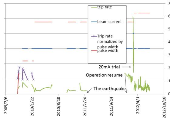
Figure 1: History of the trip rate of RFQ I from just after the vacuum improvement to the last run.
