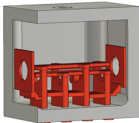
Figure 4: MWS model of the Test-RFQ
