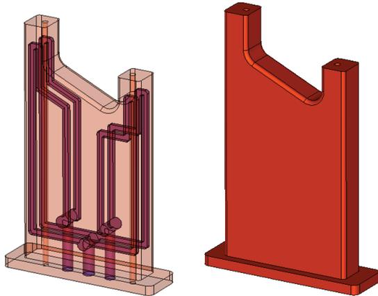
Figure 6: New stem design with the cooling channels.
