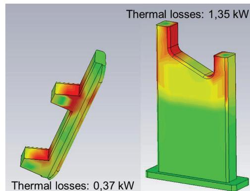
Figure 5: Current distribution and thermal losses.
