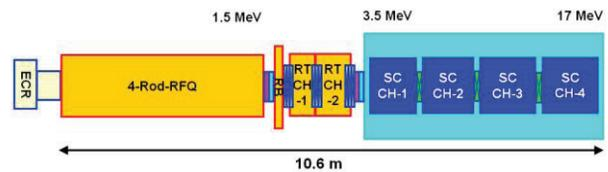
Figure 2: General layout of the MYRRHA injector.
