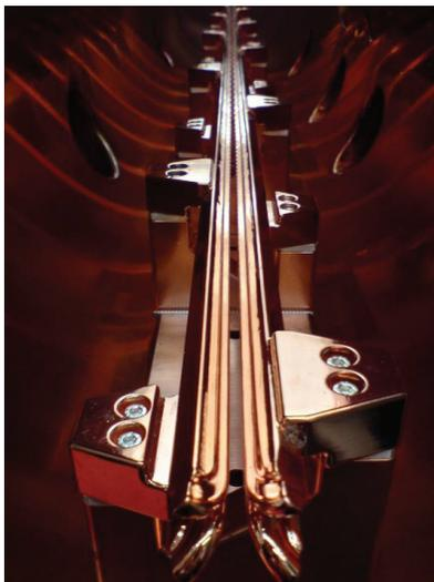
Figure 3: Picture of a typical 4-rod RFQ.
