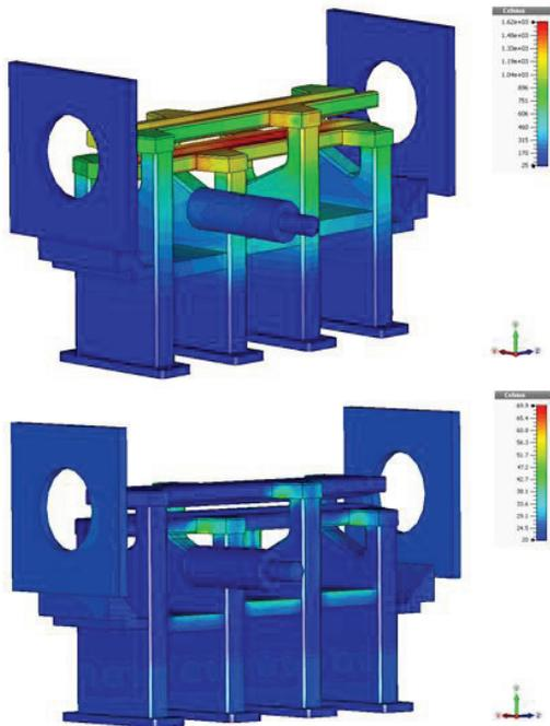
Figure 7: Thermal Microwave Studio simulations with (bottom) and without (top) cooling.
