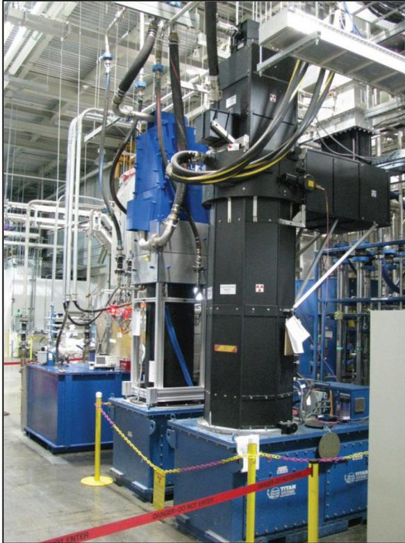
Figure 5: The existing RF test stand features a high-voltage converter modulator (background) which can be used to operate either 2.5 MW, 402.5 MHz or 5 MW, 805 MHz klystrons (foreground).
