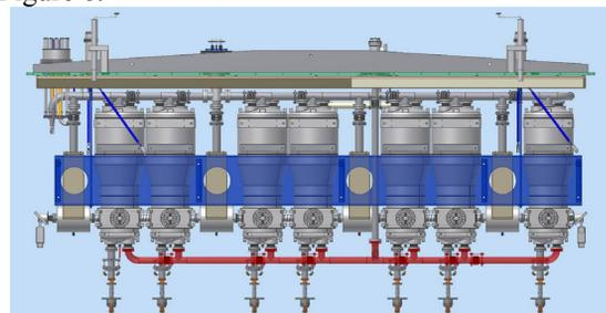
Figure 6: ANL cryomodule with five cavities and focusing solenoids.
