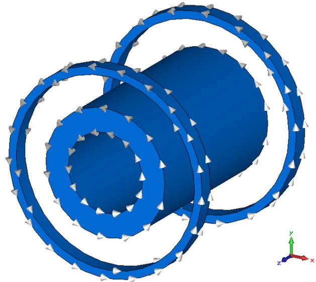
Figure 5: Main and bucking coils of the superconducting solenoid.
