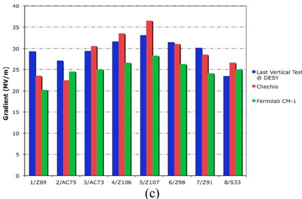
Figure 5: Field gradient achieved in cryomodules developed at (a) DESY/FLASH-PXFEL1 [7], (b) KEK/S1-Global [14], and (c) Fermilab/NML/ASTA-CM1 [10].
