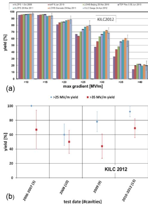
Figure 4: Progress of the ILC-SCRF 1.3 GHz cavity gradient R&D (a) integrated production yield in the 2<sup>nd</sup> pass process, with the data available since 2006, and (b) differential production yield. [9]. The blue points are for >25 MV/m yield and red points are for >35 MV/m yield.
