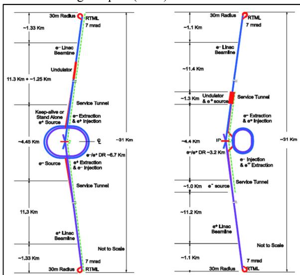
Figure 1: Layouts of ILC in RDR (left) and TDR (right).
