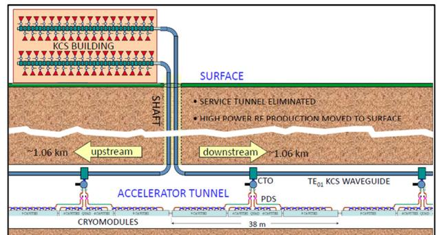
Figure 6: The KCS concept for the main linac HLRF power distribution system considered in flat-land site topography.
