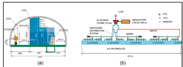
Figure 7: The DKS concept for the main linac HLRF power distribution system considered in mountainous site topography finalized in TDR.
