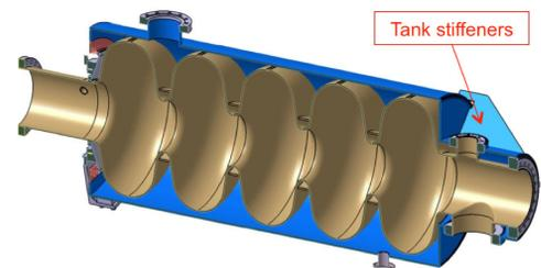
Figure 5: A cross-section through a high- $\beta$  elliptical cavity installed within its cryo-vessel.
