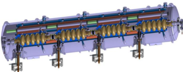
Figure 3: Elliptical cavity cryomodule for ESS
