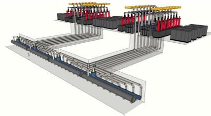
Figure 6: The ESS RF sources in stub lay-out
