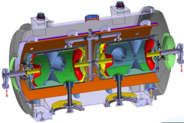
Figure 2: Spoke cavity cryomodule for ESS
