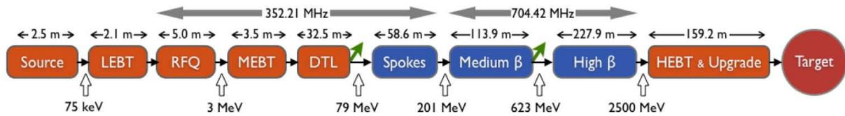
Figure 1: A block diagram of the ESS linac design. The Radio Frequency Quadrupole (RFQ) and Drift Tube Linac (DTL) are normal conducting while the spoke resonator and low beta and high beta elliptical cavities are superconducting
