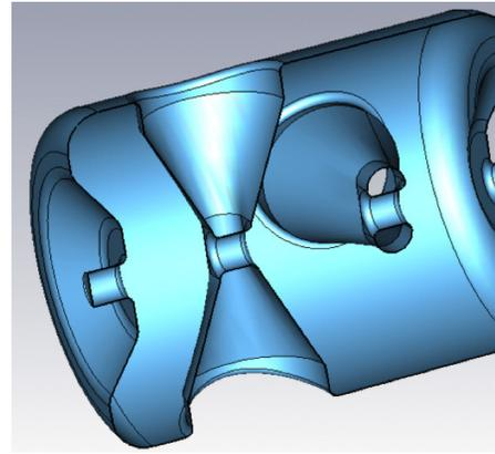
Figure 4: A cross-section through a spoke cavity design for ESS.
