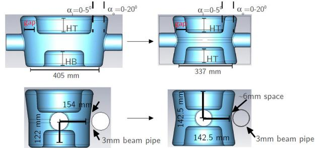
Figure 9: Asymmetric and symmetric 400 MHz quarter-wave crabbing cavities.
