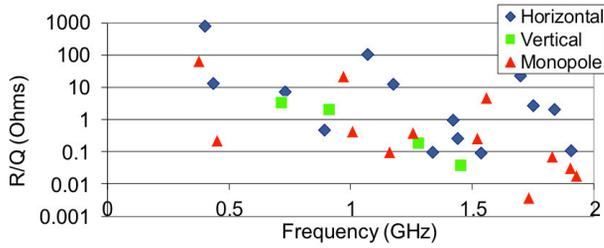
Figure 6: HOM spectrum of the 4-rod crabbing cavity.
