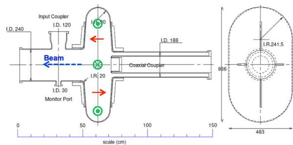
Figure 2: Superconducting 508.9 MHz KEK crabbing cavity.
