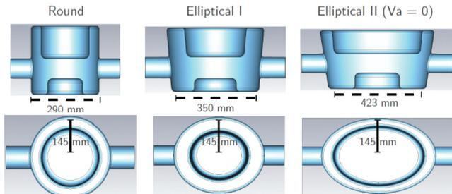
Figure 7: Superconducting 400 MHz quarter-wave deflecting/crabbing cavity by BNL.
