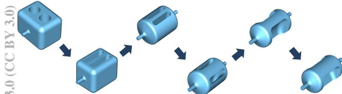
Figure 11: Design evolution of the parallel-bar cavity into the rf-dipole cavity.
