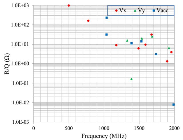
Figure 14: HOM spectrum of the 499 MHz rf-dipole cavity.
