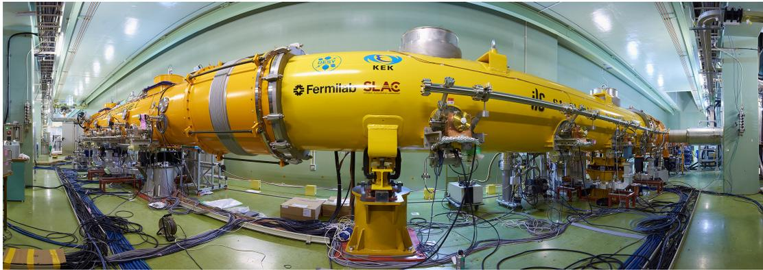
Figure 1: The S1-Global cryomodule from the view of the input coupler side. Right cryomodule is from INFN.
