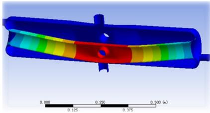
Figure 5: One of Model analyses results of HWR cavity with cleaning pipes free ( cavity deformation).
