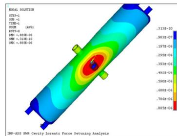
Figure 4: Deformation of the cavity wall (fix boundary condition)
