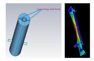
Figure7: Supporting rods on the short plate (left); deformation of ring-and-supporting-rods-stiffened QWR by external pressure: df/dP~-29 Hz/mbar.
