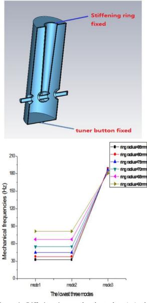
Figure 4: Stiffening ring on the short plate (up); the lowest three vibration modes frequency on the dependence of the radius of stiffening ring (down).
