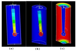
Figure 5: The lowest three vibration modes for stiffened-ring with radius 60mm QWR cavity.
