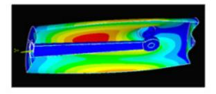
Figure 6: Deformation of ring-stiffened QWR caused by the external pressure, the frequency shift  $\Delta f$  due to the change in ambient pressure  $\Delta P$ : df/dP~-37 Hz/mbar.
