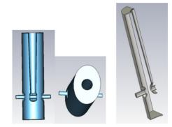
Figure 1: Mechanical model of the elliptical cylinder outer conductor QWR for the structural analysis.
