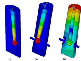
Figure 3: The lowest three vibration modes for the new-shaped naked QWR cavity.
