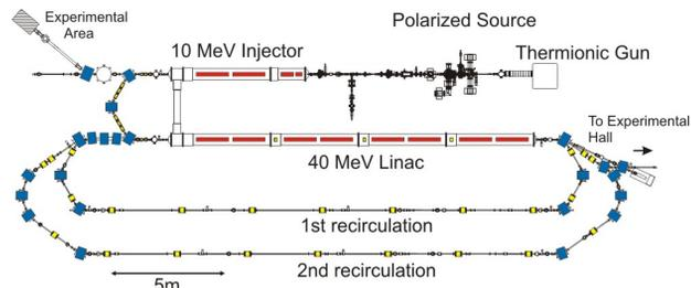
Figure 1: Floor plan of the S-DALINAC.
