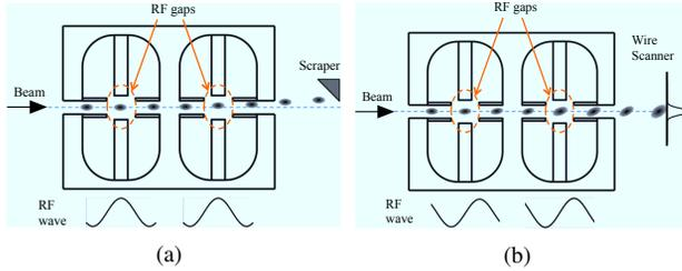
Figure 2: The RF setting and a beam bunch behavior — (a) In the nominal operation (b) In the measurement.
