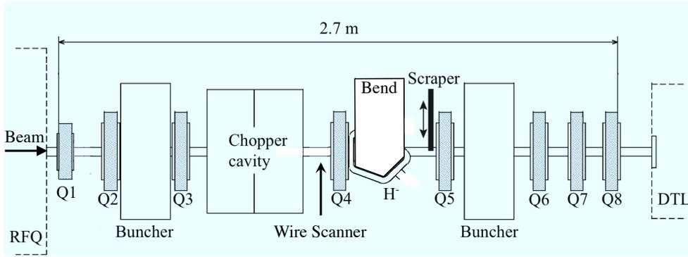
Figure 1: Layout of MEBT1. We use the chopper cavity, the upstream buncher cavity and the wire scanner between the chopper cavity and Q4 for the measurement.
