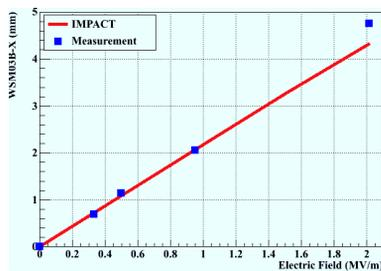
Figure 3: Correlation of the chopper electric field and the deflection at the WSM.
