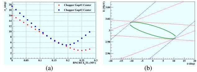
Figure 4: The simulation results — (a)  $\sigma_\phi$  at both RF gaps of the chopper as a function of the buncher  $E_0TL$  (b) The ellipse and the boundaries obtained by  $\sigma_\phi^C$  measurement. The dotted lines are the boundary at 0 (red), 0.085 (magenta) and 0.17 MV (blue), respectively.
