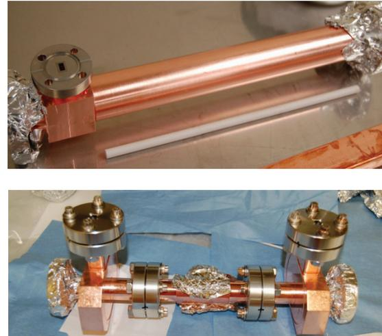
Figure 5: 26 GHz power extractor and accelerating structure.
