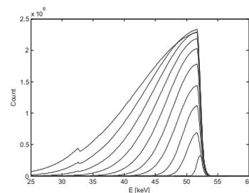
Figure 8: The x-ray spectrum with different collecting angle.
