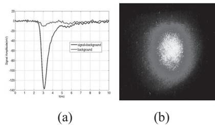
Figure 2: typical X-ray signal and background from the MCP detector(a) and X-ray CCD.
