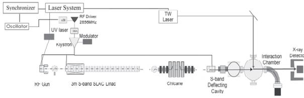
Figure 1: scheme of TTX.
