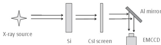
Figure 5: The scheme of the X-ray spectrum measurement.
