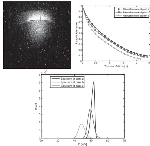
Figure 6: (top left) X-ray profile measured by EMCCD sheltered by 1.5cm silicon. (top right) Attenuation curves at points a, b, and c. (bottom) The reconstructed local X-ray spectrum from the attenuation curves.
