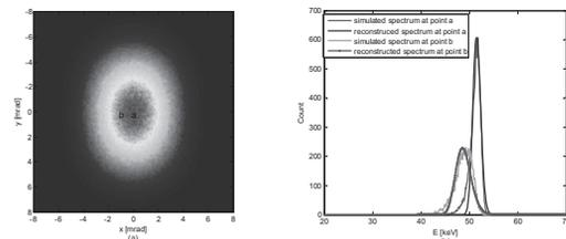
Figure 3: (a) X-ray profile simulated by CAIN and the two points selected to reconstruct local spectra. (b) Simulated and reconstructed spectra at two different points with 0.5 mrad collecting angles and 5% Gaussian random error.
